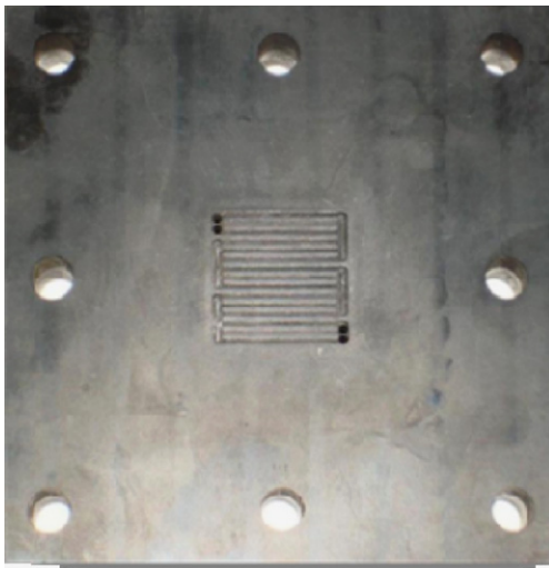
Fig. 1. Experimental monopolar plate (EFC05-01SP) with serpentine flow-field.
